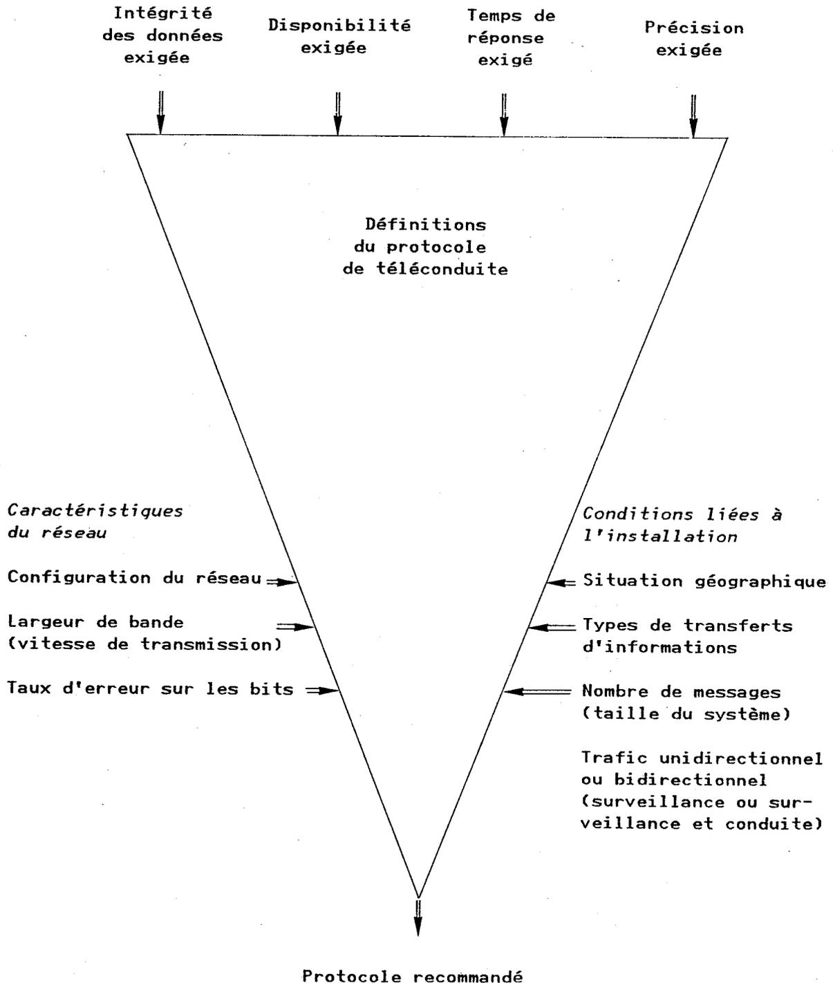
Data transport is only one function of the total system. The speed and integrity requirements of data transmission shall be chosen to be consistent with the accuracy of the total system, i.e. all the system parameters should be matched. In addition to the required compromise between transmission speed and transmission integrity there are further conditions which influence the choice of an appropriate telecontrol protocol, as shown in the following diagram:
